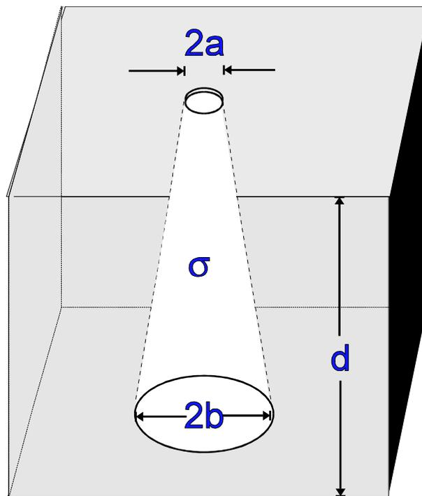
Fig. 1. A conical nanopore in a portion of insulating membrane of thickness  $d$ . The nanopore is filled with a liquid of conductivity  $\sigma$ , which also bathes both faces of the membrane. In a particle-measuring application, the membrane would be semi-infinite in extent and contacted by "O"-rings so that the two sides are electrically isolated from each other.
