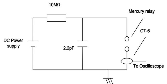
Fig. 1 Electrical circuit for low voltage ESD experiment.
