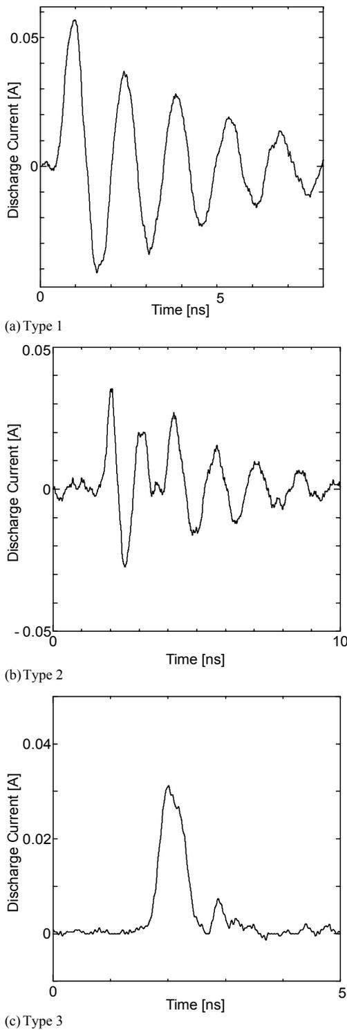
Fig. 6 Current wave form at 10 V.
