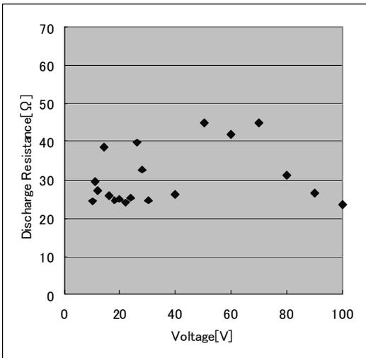
Fig.9 (b) Resistance of the switching area V is less than 100V
