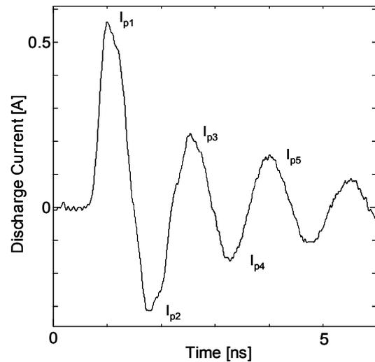
Fig.5 A discharge current waveform (50V)
