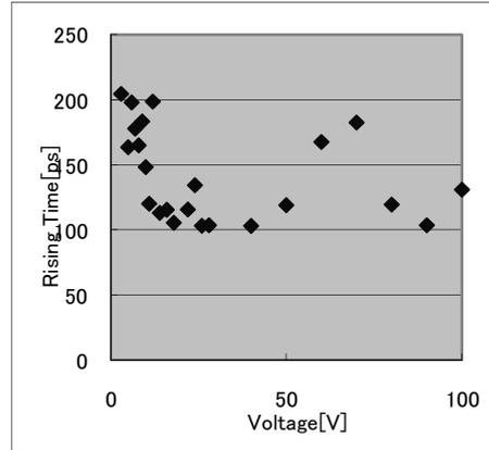
Fig.10 Peak current rising time versus charging voltage.
