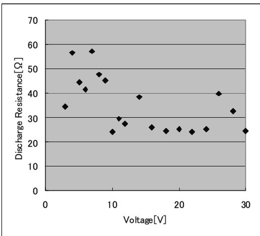
Fig. 9 (a) Resistance of the switching area V is less than 30V.
