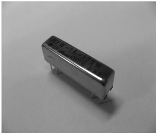
Fig.2 A photo of mercury reed switch
