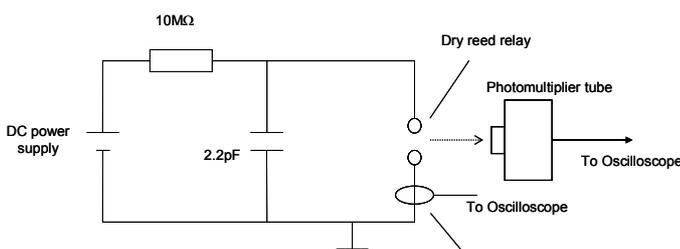
Fig.4 Optical emission measurement of low voltage ESD
