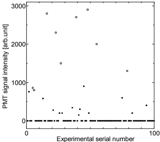
Fig.11 Optical output (photomultiplier output) intensity for repeated process where the charging voltage of the capacitor is 160 V.
