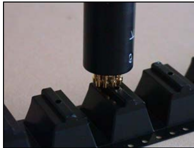
Fig. 6 Measurement of a blister belt with a small ring probe
