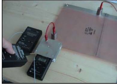
Fig. 7 Simple test method for static decay time
