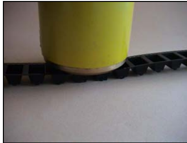
Fig. 5 Measurement of a blister belt with a normal probe
