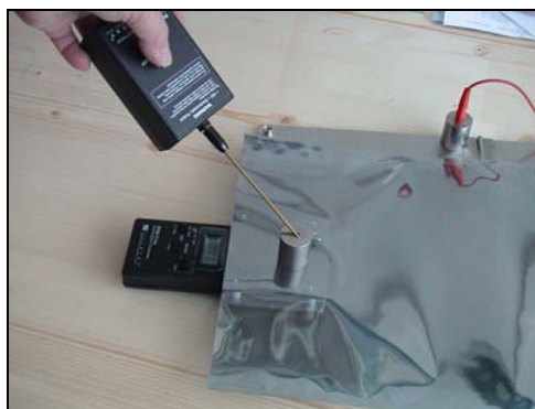
Fig. 8 Simple test method for shielding property
