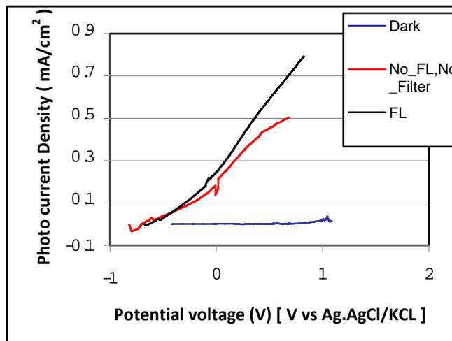
Fig. 1. Photocurrent density of TiO<sub>2</sub> photoanode. The plot shows dark current, current with light source, and with light source and Fresnel Lens.
