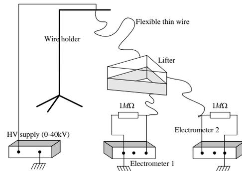
Fig. 16 Set up for the levitation experiment
