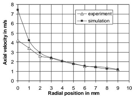
Fig. 4. Numerically calculated and experimental axial velocity profiles 3.6 cm away from the tip of 95 μm needle 2cm above the grounded metal grid at 13 kV.
