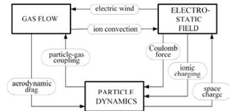
Fig.12 Fields and their interactions during the precipitation process
