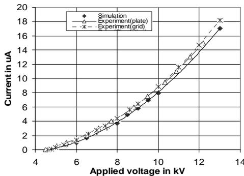
Fig. 3. Calculated and experimental I-V characteristics for metal grid and plate as a cathode.
