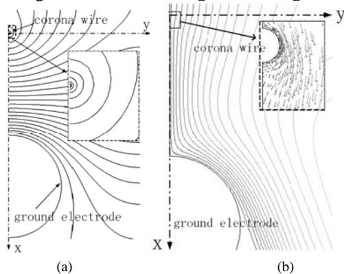
Fig. 19 (a) Equipotential lines in the levitation device and (b) the airflow pathlines between both electrodes.
