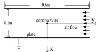
Fig. 13 Two-dimensional computational model of a wire-plate ESP
