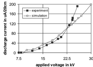
Fig. 20 Comparison of experimental and calculated  $I-V$  characteristics
