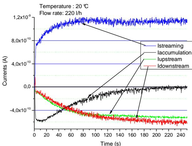
Fig. 2. Typical currents measured on the sensor for "low leakage impedance" configuration.
