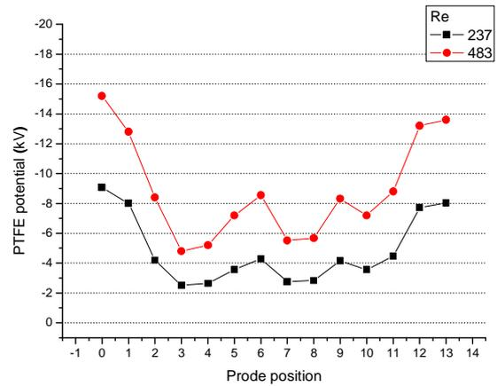
Fig. 11. Map of P.T.F.E. electric potential for used oil and duct without obstacles for different Reynolds numbers
