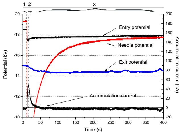
Fig. 12. Potential and current measurements versus times (Re 237)
