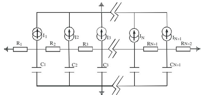
Fig. 3. Electrical analogical circuit proposed to model flow electrification phenomenon on dielectric solid surface.  $I_N$  are the different current generators and  $R_N$  the leakage resistances and  $C_N$  the capacitive values distribute all along the duct.
