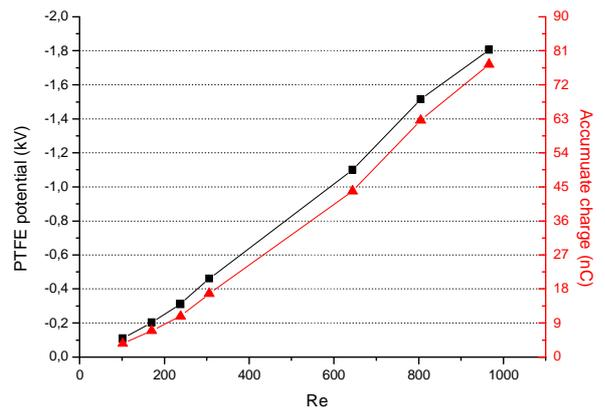
Fig. 8. P.T.F.E. potential measurement and accumulate charge versus Reynolds number.
