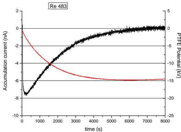
Fig. 7. Correlation between accumulation current and P.T.F.E. potential measurements versus time for constant Reynolds number Re 483. Accumulated charge :  $1.56 \cdot 10^{-6} \text{ C}$ .
