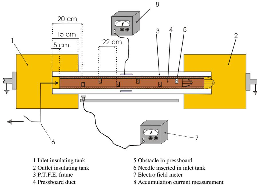
Fig. 6. The new configuration device for study electrostatic hazards
