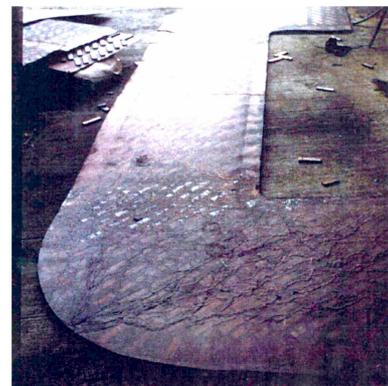
Fig. 1. Electrostatic discharge at pressboard surface coming from damage power transforming.
