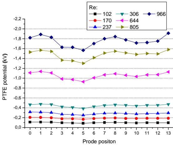
Fig. 9. Map of PTFE electric potential for new oil and duct without obstacles for different Reynolds numbers.
