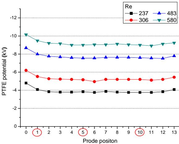
Fig. 10. Map of PTFE electric potential for new oil and duct equipped with obstacles for different Reynolds numbers. Probe positions 1, 5 and 10 are corresponding to position of the flow obstacles.
