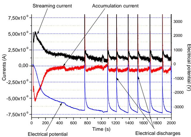
Fig. 5. Inlet tube potential, accumulation and streaming currents for “high leakage impedance” configuration.
