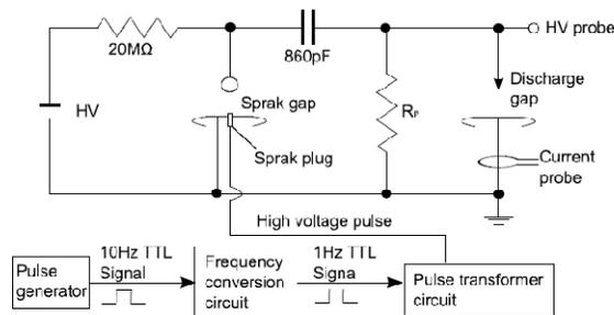
Fig. 1. High voltage circuit
