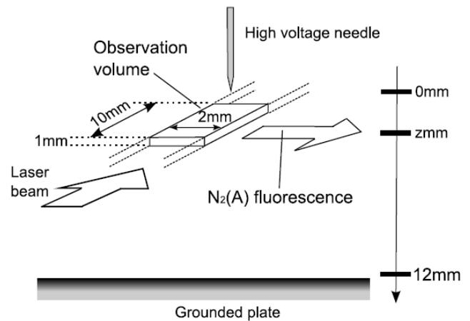
Fig. 3. Beam path and observation volume for LIF measurement.
