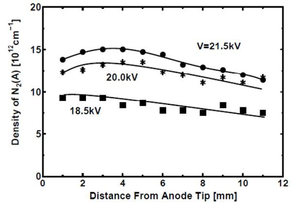
Fig. 7 one-dimensional distribution of  $N_2(A^3\Sigma_u^+)$
