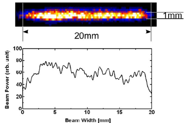
Fig. 4 Cross section of laser beam and one-dimensional distribution of laser intensity
