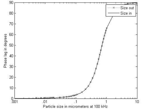
Fig. 4. Semilog graph of phase lag versus particle size for 100 kHz exciting frequency
