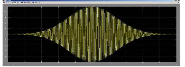
Fig. 1. Doppler burst formed by Gaussian shape and signal model
