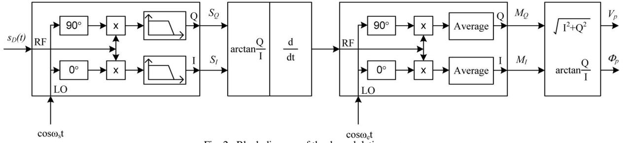
Fig. 2. Block diagram of the demodulation process
