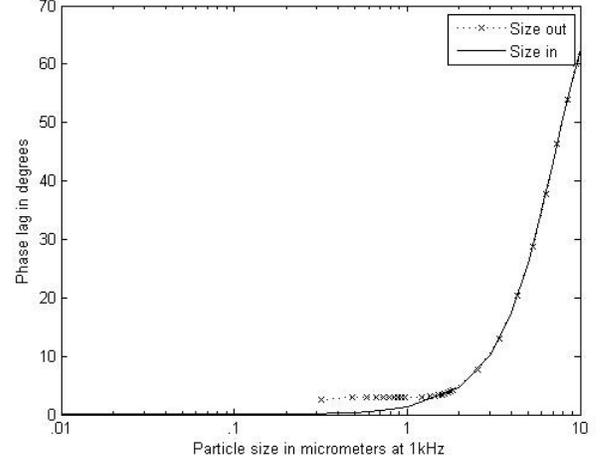
Fig. 3. Semilog graph of phase lag versus particle size for 1 kHz exciting frequency
