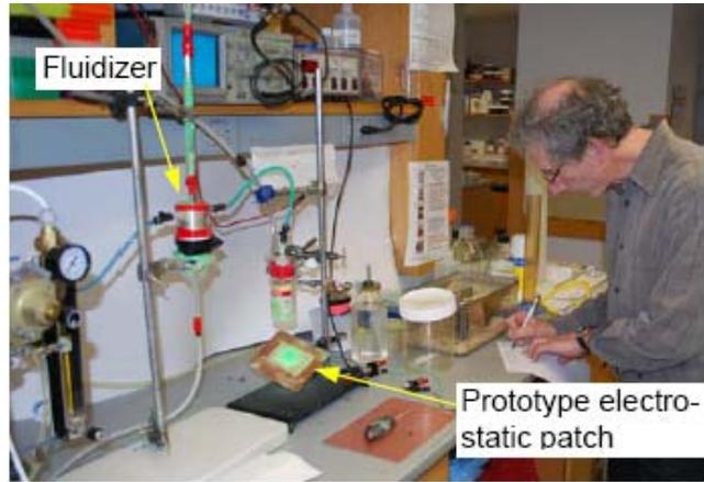
Figure 3 – Particle charging apparatus in the laboratory.
