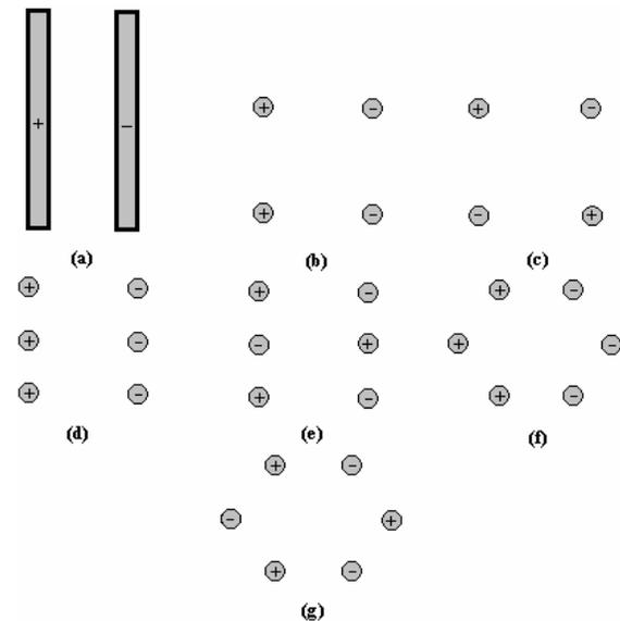
Fig. 3. Electrodes shapes and arrangements (a) Parallel plate electrode (b) Four-needle electrode with positive voltage on one side (c) Four-needle electrode with positive voltage at diagonal position (d) Parallel six-needle electrode with positive voltage on one side, (e) Parallel six-needle electrode with positive voltage at alternation (f) Six-hex-needle electrode with positive voltage on one side (g) Six-hex-needle electrode with positive voltage at alternation.
