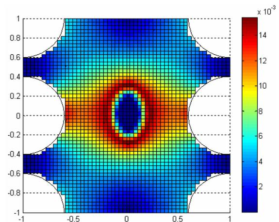
Fig. 11. The electric field distribution of the elliptical cell with 90° rotation in the parallel six-needle electrode
