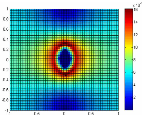
Fig. 8. The electric field distribution of the elliptical cell with 90° rotation in the parallel plate electrode
