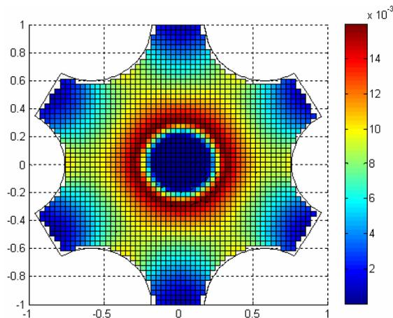
Fig. 6. The intensity distribution of the round cell in the six-hex-needle electrode
