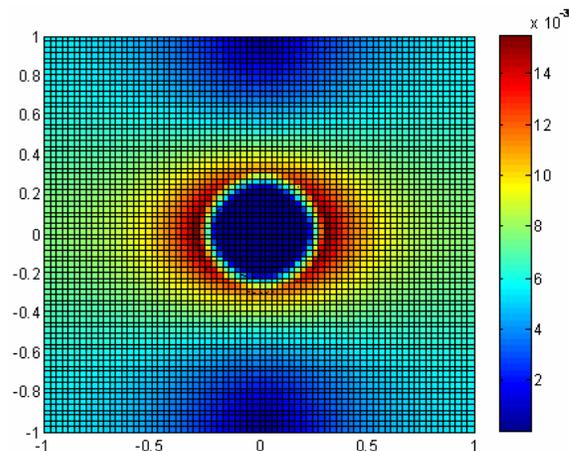
Fig. 4. The intensity distribution of the round cell in the parallel plate electrode
