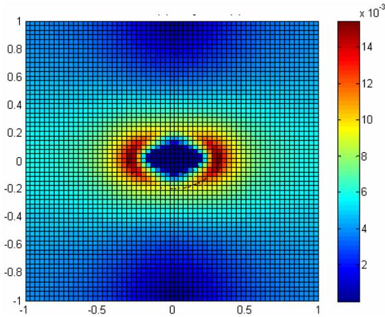
Fig. 7. The electric field distribution of the elliptical cell in the parallel plate electrode
