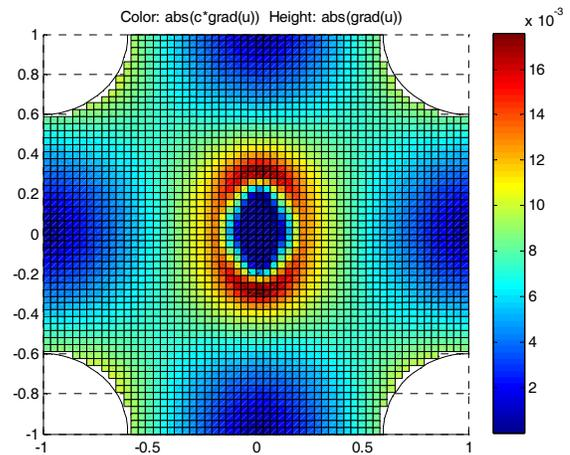
Fig. 9. The electric field distribution of the elliptical cell with 90° rotation in the four-needle electrode
