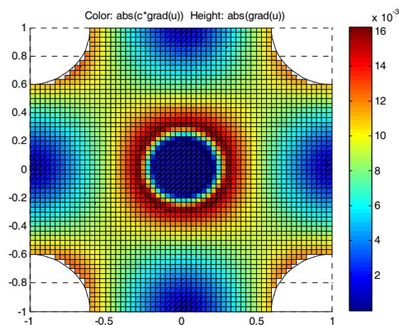
Fig. 5. The intensity distribution of the round cell in the four-needle electrode
