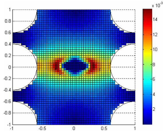
Fig. 10. The electric field distribution of the elliptical cell in the the parallel six-needle electrode
