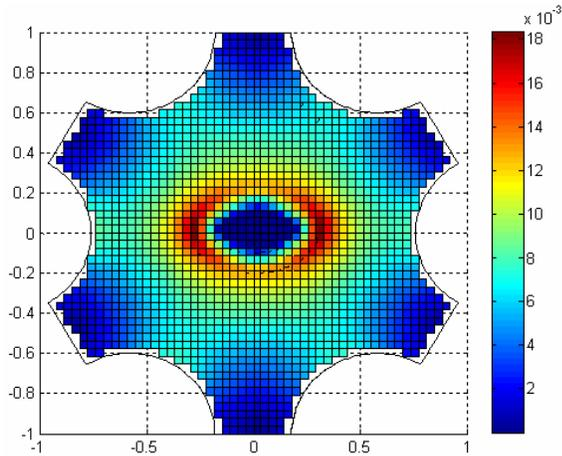
Fig. 12. The electric field distribution of the elliptical cell in the six-hex-needle electrode
