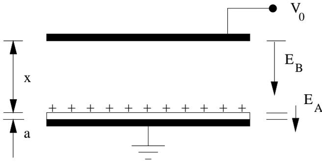
Fig. 3. Electric field model for capacitive MEMS structure
