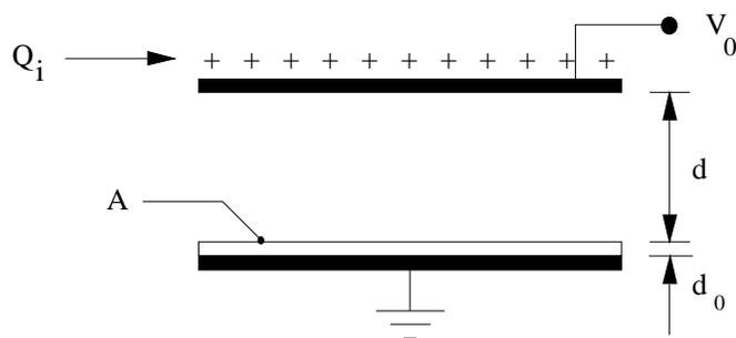
Fig. 1. Parallel plate model for capacitive MEMS
