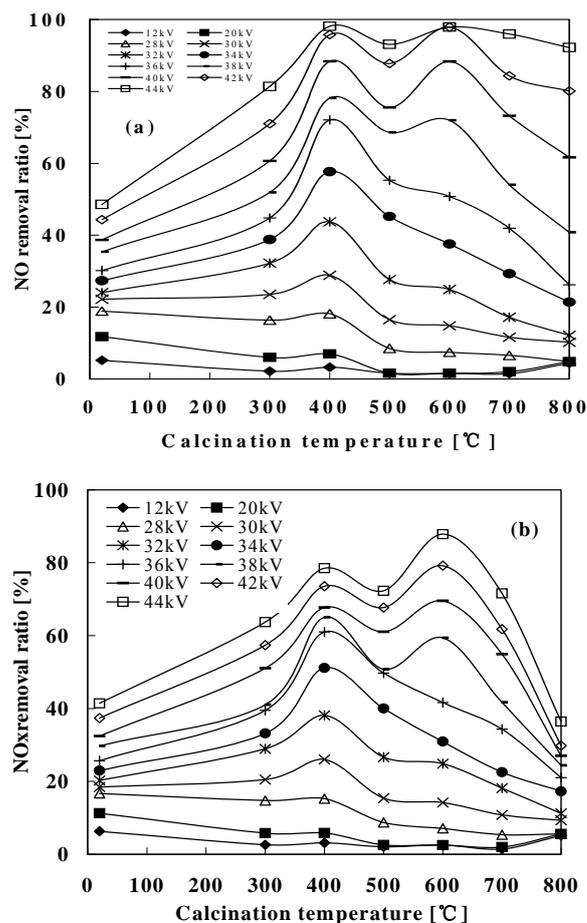
**Fig. 4 The co-relation between MAC calcination temperature and (a) NO and (b)NO<sub>x</sub> removal ratios for various discharge voltage**
