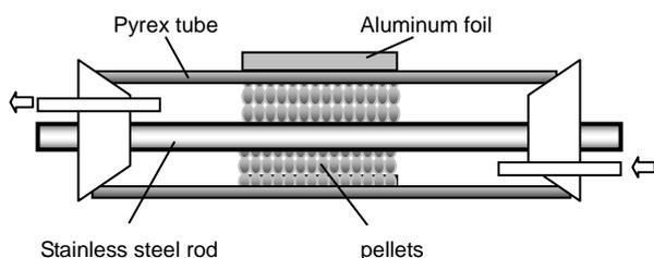
**Fig.1 reactor structure**
