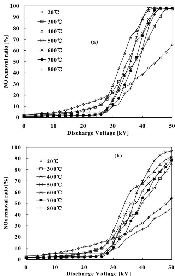
**Fig.3 NO(a) and NO<sub>x</sub>(b) removal ratio versus discharge voltage**
