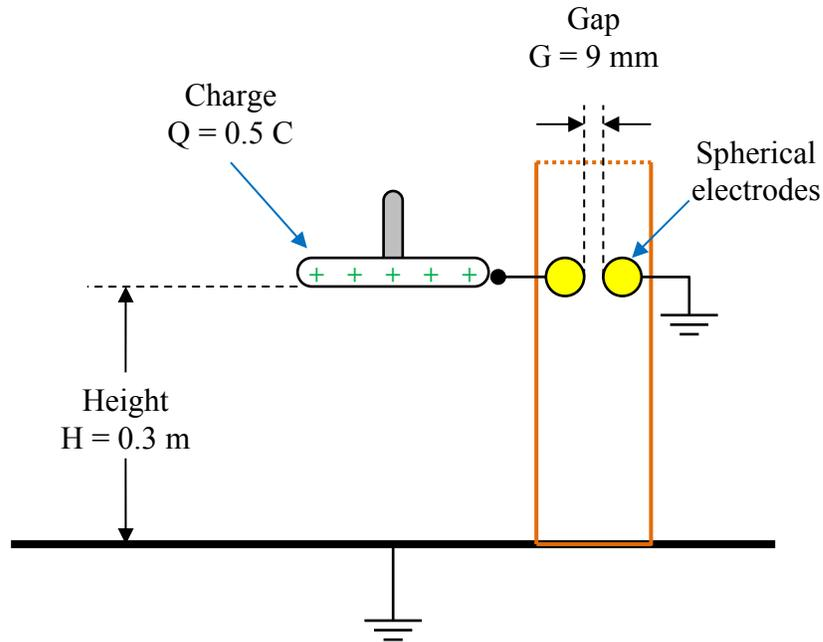
Figure 2: Lifting the charged, isolated electrode increases the stored electrical energy. Touching the charged electrode to the isolated spherical electrode releases the stored energy in a spark.
