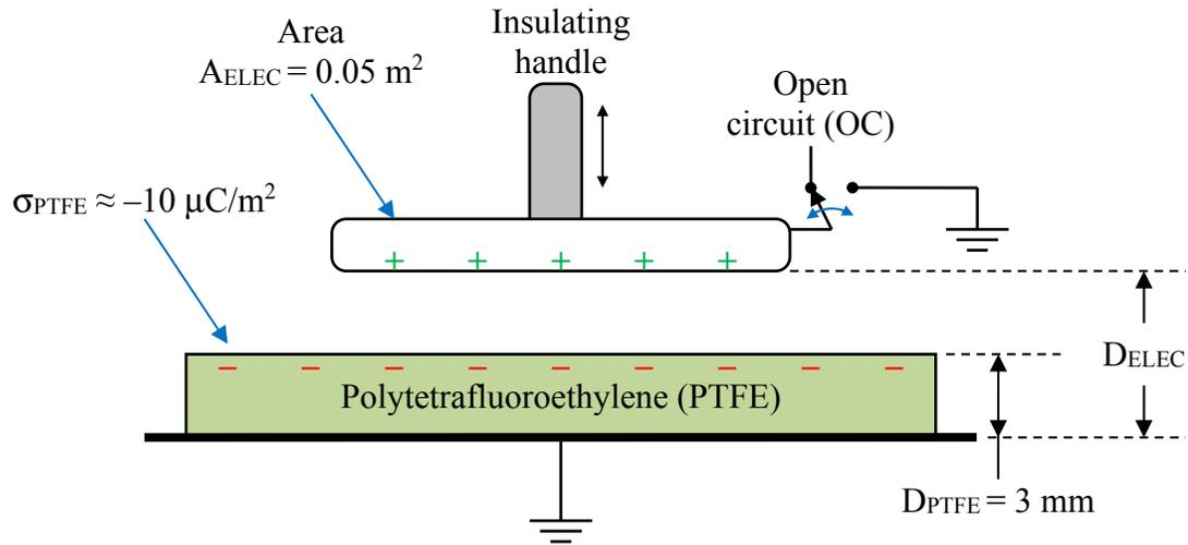
Figure 1: Static charge is induced on the electrically isolated electrode by placing it in contact with the charged PTFE and temporarily closing the switch to ground.
