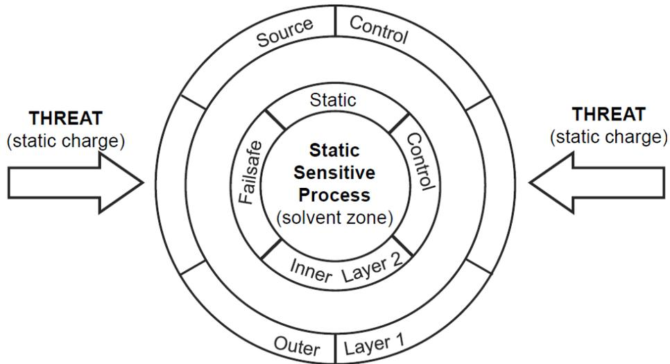
Figure 1: Two layers of static dissipaters protect risks from threats.
