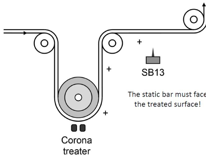
Static bar SB13 neutralizes charge on the treated surface from the corona treater.
