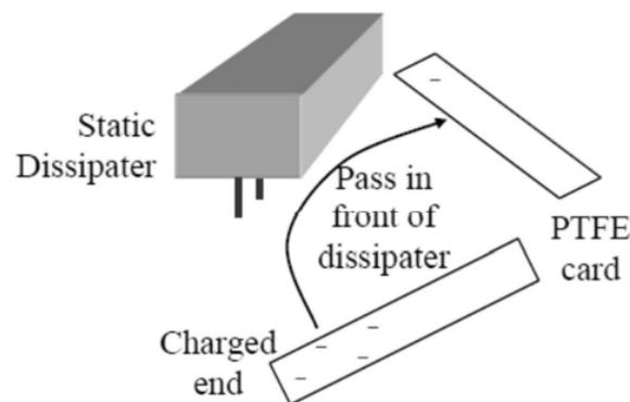
Figure 12: Test the neutralization efficiency of a static dissipator by measuring the reduction in static charge on a piece PTFE (of other polymer) using a hand held fieldmeter.
