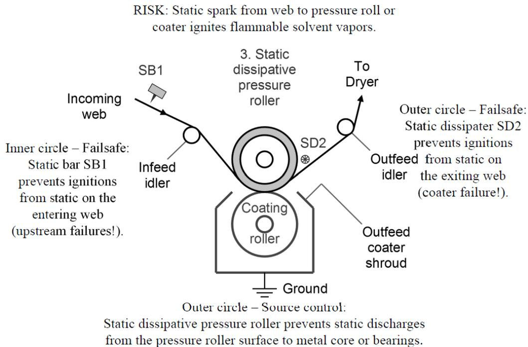
Figure 8: Static control for solvent coaters have 3 elements.
