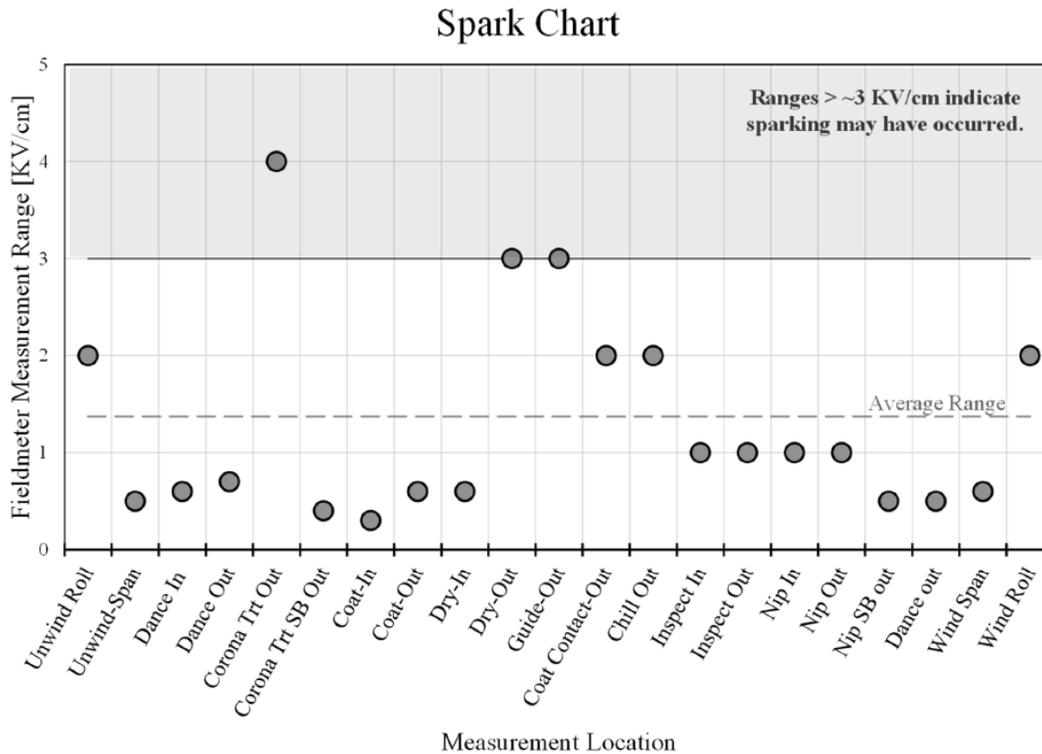
Figure 7: Plot the range of readings to find where sparks have occurred.
