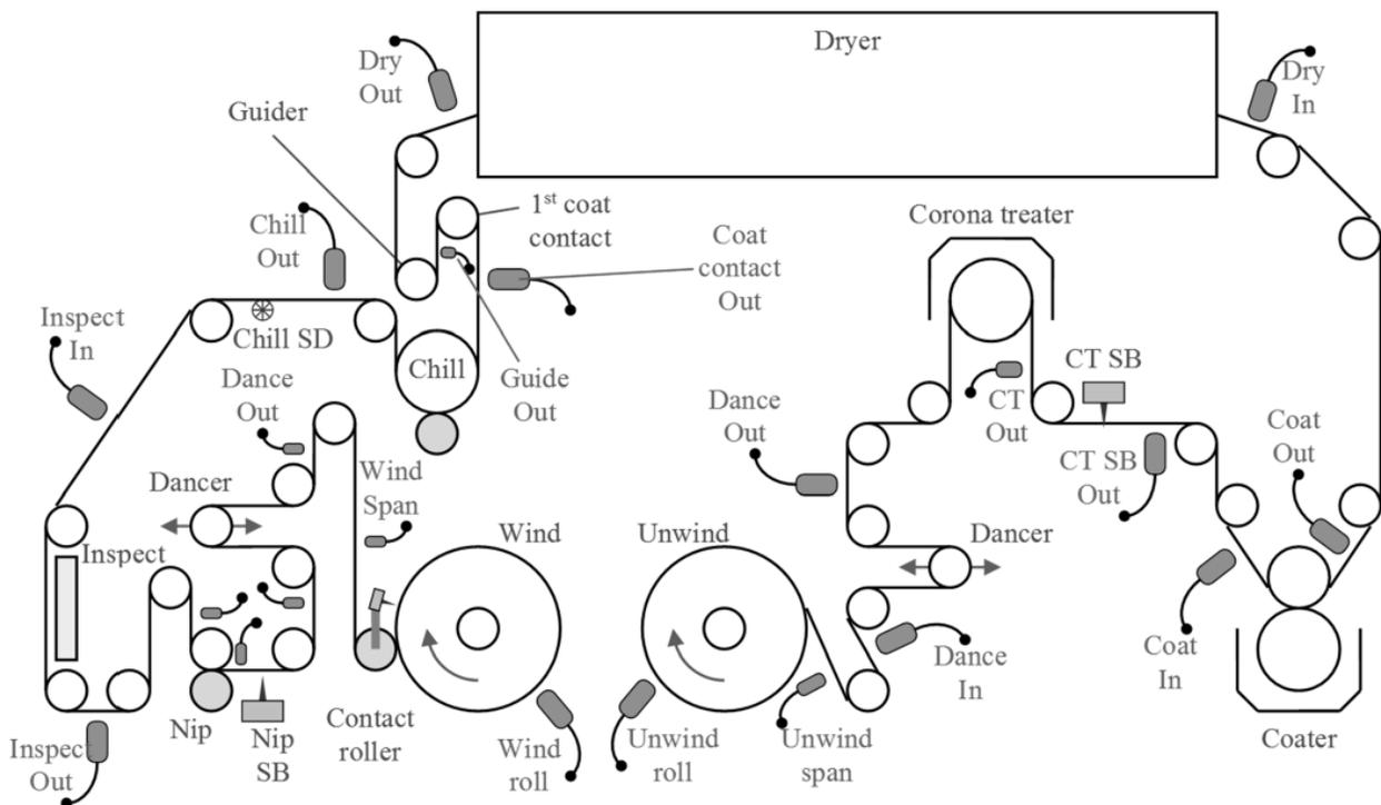
Figure 2: Measure the electric field on each accessible web span.
