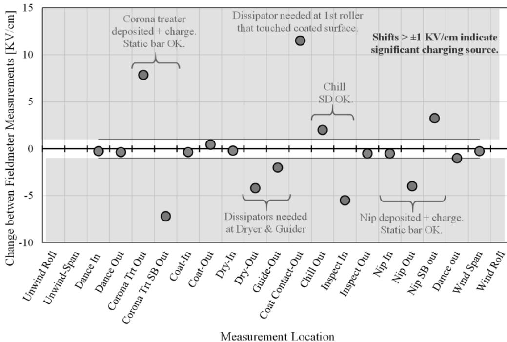
Figure 6: Plot the shift in the readings to identify sources of static charging.
