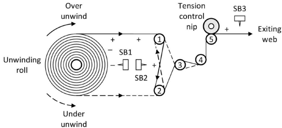
Static is neutralized on both sides of the web exiting the unwinding roll.
